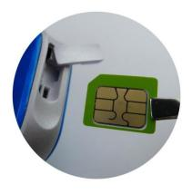
2. Insert the SIM card completely
